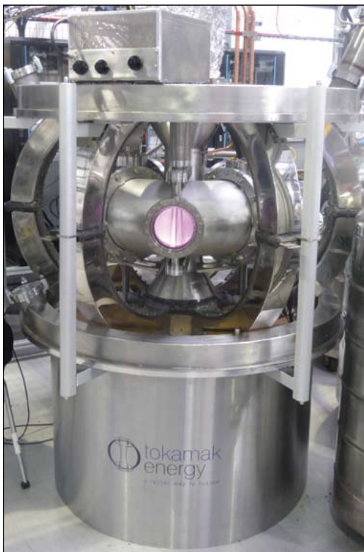
The ST25 with high temperature superconductors. High temperature superconducting magnets could be used to create high magnetic fields in a compact spherical tokamak
